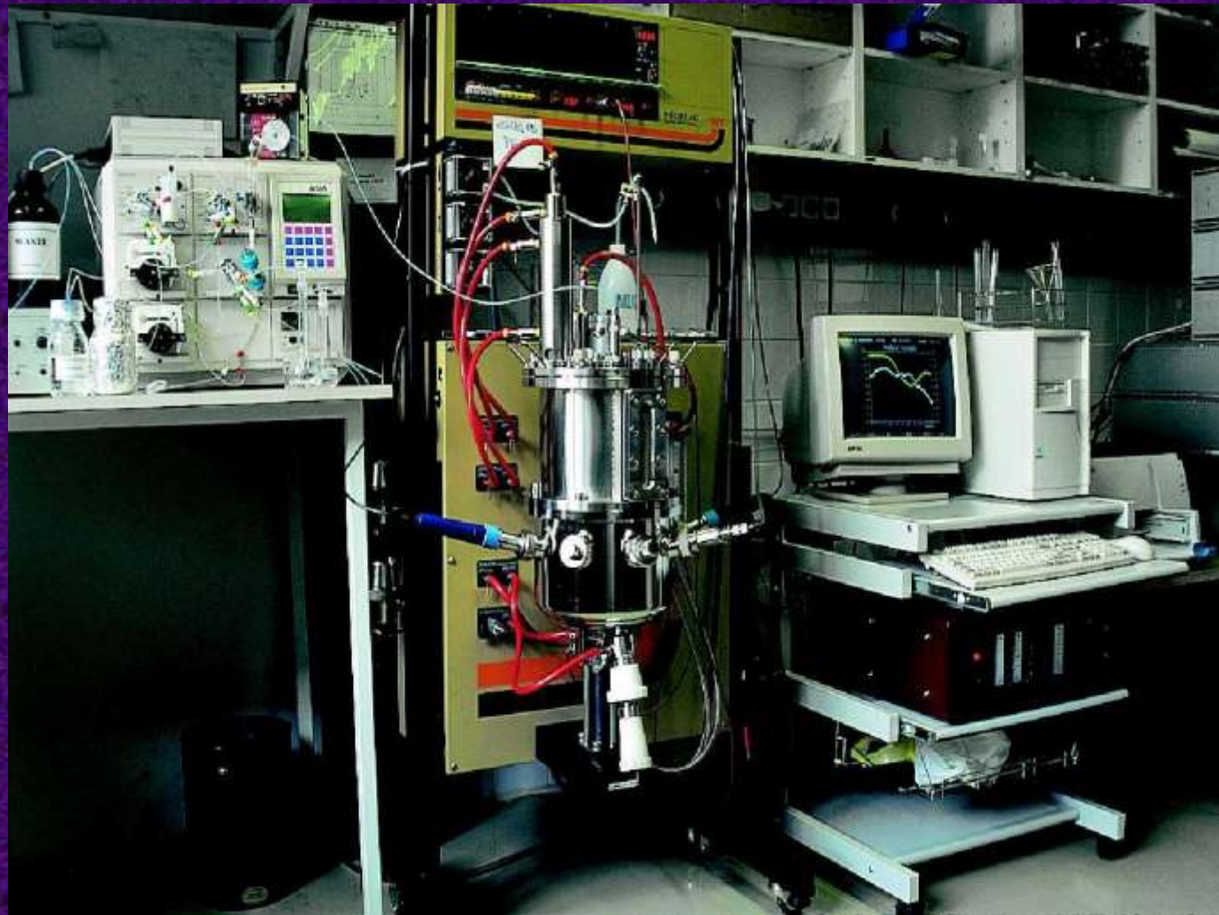
Stirred Tank Reactor and instrumentation for on-line process control
